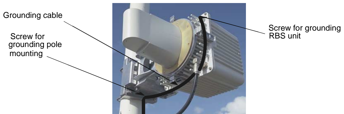
Figure 34 – Grounding the outdoor equipment with the 9900UX1102 pole mounting
