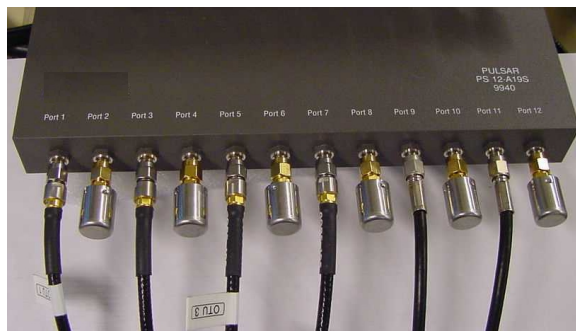
Figure 20 – Connecting the Bias-T to the Combiner/Splitter
