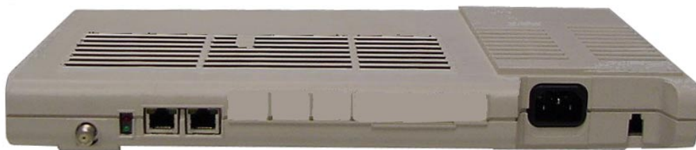
Figure 16 – Earthing the (NCFxxx) NT Lite unit
