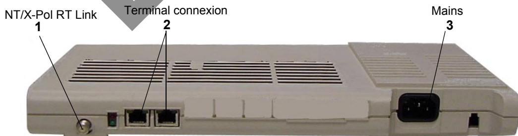
Figure 23 – The NT Lite unit (85 – 264 V \sim 47 – 63 Hz)
