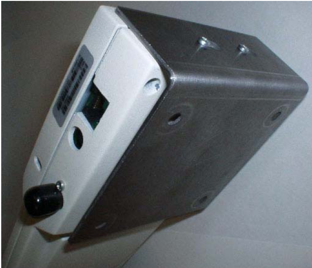
Figure - Assembling the OmniAccess AP to the Flush-Mount Bracket
