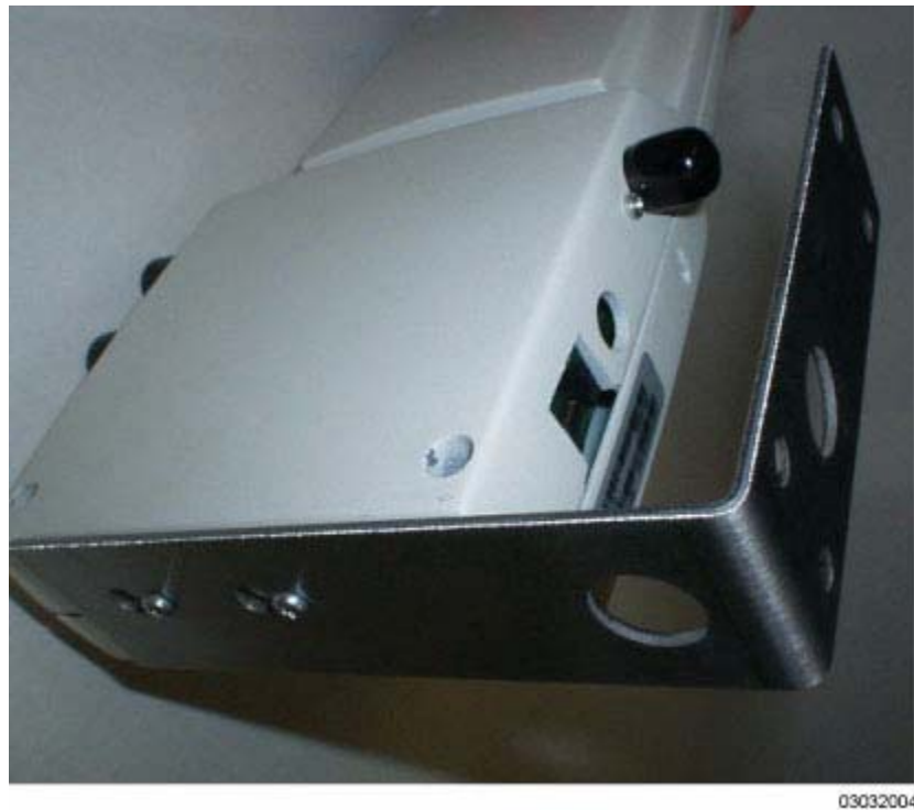
Figure - Assembling the OmniAccess AP to the Projection-Mount Bracket
