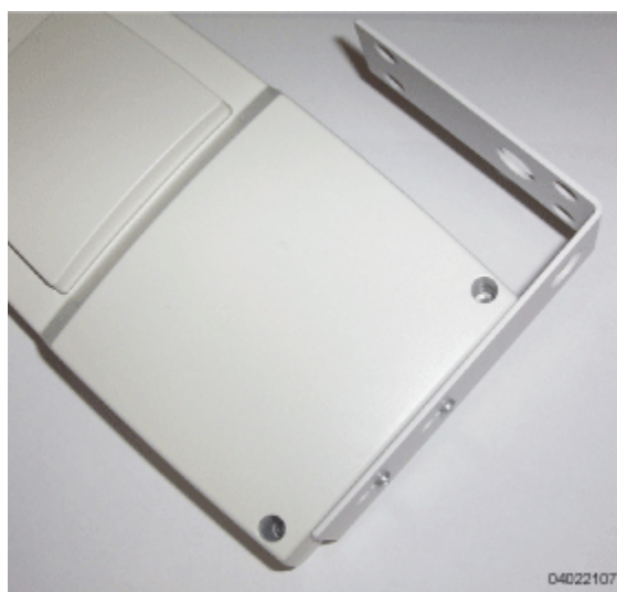
Figure - Assembling the OmniAccess AP to the Projection-Mount Bracket
