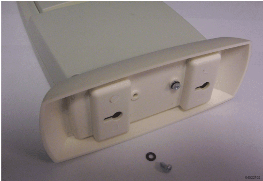
Figure - Assembling the OmniAccess AP and Ceiling-Mount Base
