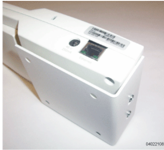
Figure - Assembling the OmniAccess AP to the Flush-Mount Bracket
