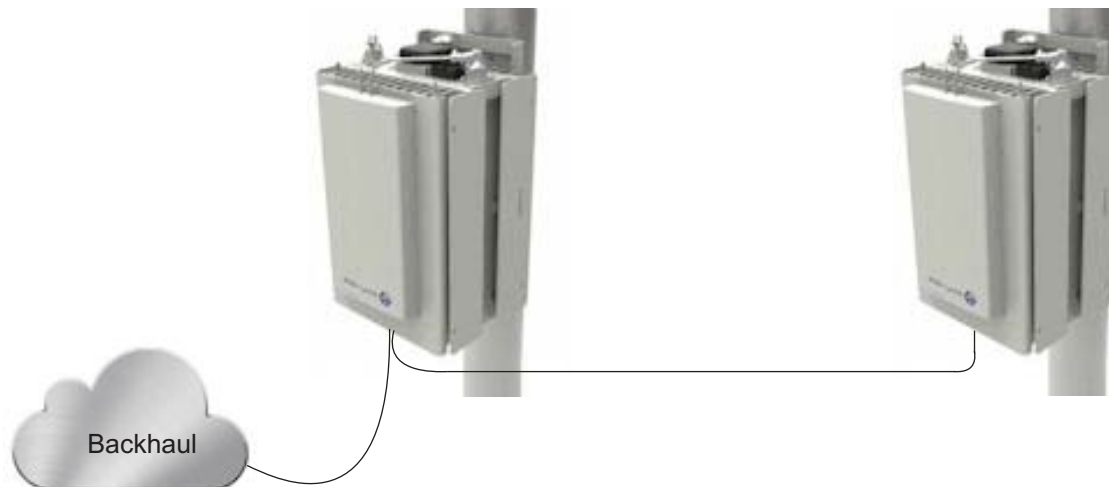
Figure 2-6 9764 MCO daisy chain installation example
