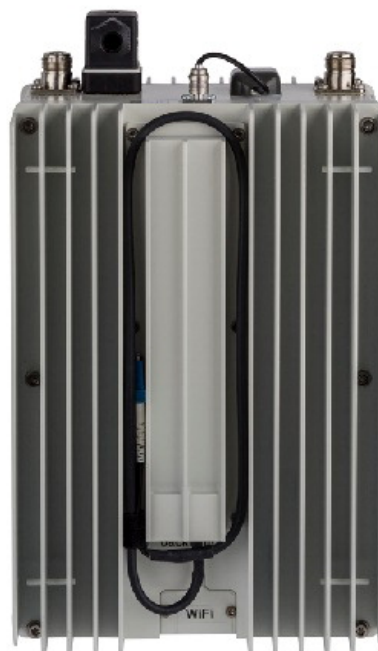
back view with the RF components and Baseband Unit into the 9764 CMCO module
