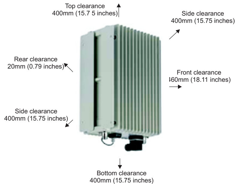
Figure 3-2 9768 CMRO installation clearances
