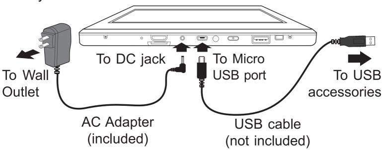
**Note:** Micro USB port for charging at either OFF mode or Standby mode.
