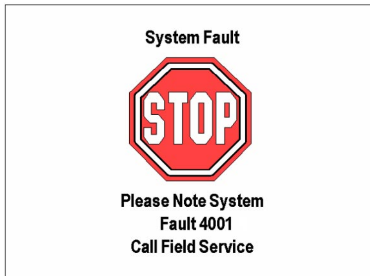
Figure 5-1 System Fault Display Screen
