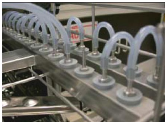
Figure 4-3. Auto Wash: Unused Injectors Shown Plugged Off Pictured: Miele* Labwasher, Model G7735 with injector Model #0-177
