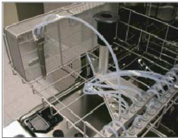
Figure 4-2. Auto Wash: "Y" Adapter Connected to Injector Nozzel
