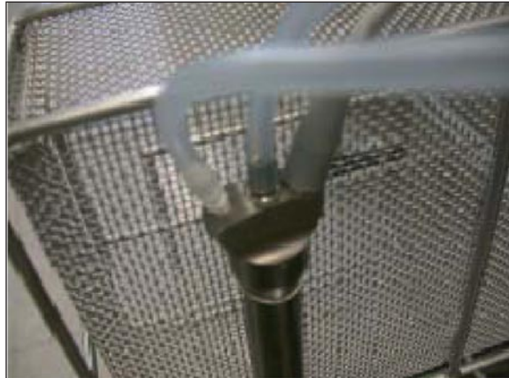
Figure 4-1. Auto Wash: Handpiece with "Y" Adapter Connected
