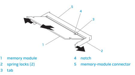
To replace the memory modules, perform the removal steps in reverse order. While inserting the memory module into the connector align the notch on the memory module with the tab on the memory module connector.
