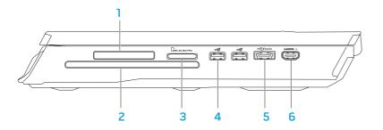
1 ExpressCard slot — Provides support for additional memory, wired and wireless communications, multimedia, and security features. The slot supports 54 mm Express cards.
