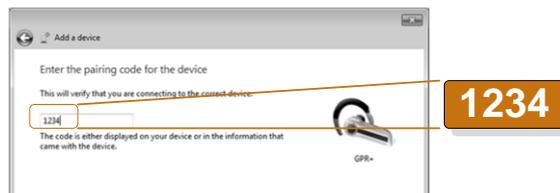
**NOTE:** If the reader is configured with Bluetooth Authentication option enabled, the pairing process is based on a code generated automatically. In this case, click next to continue (the code will not appear on the reader)
