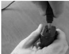
**3** Plug the adaptor into power outlet. The battery level icon will flash while charging and stop flashing when fully charged. A full charge will take approximately 3 hours.
