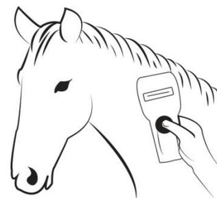
To search for microchips, press and hold down the SCAN button. The reader will display "SEARCHING" until a microchip is found or the scan button released.
