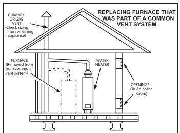
If this gas furnace replaces a furnace which was commonly vented with another gas appliance, the size of the existing vent pipe for that gas appliance must be checked. Without the heat of the original furnace flue products, the existing vent pipe is probably oversized for the single water heater or other appliance. The vent should be checked for proper draw with the remaining appliance.
