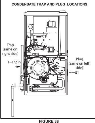
Condensate line must slope downward away from the trap to drain. If drain level is above condensate trap, condensate pump must be used. Condensate drain line should be routed within the conditioned space to avoid freezing of condensate and blockage of drain line. If this is not possible, a heat cable kit may be used on the condensate trap and line. Heating cable kit is available in various lengths:
