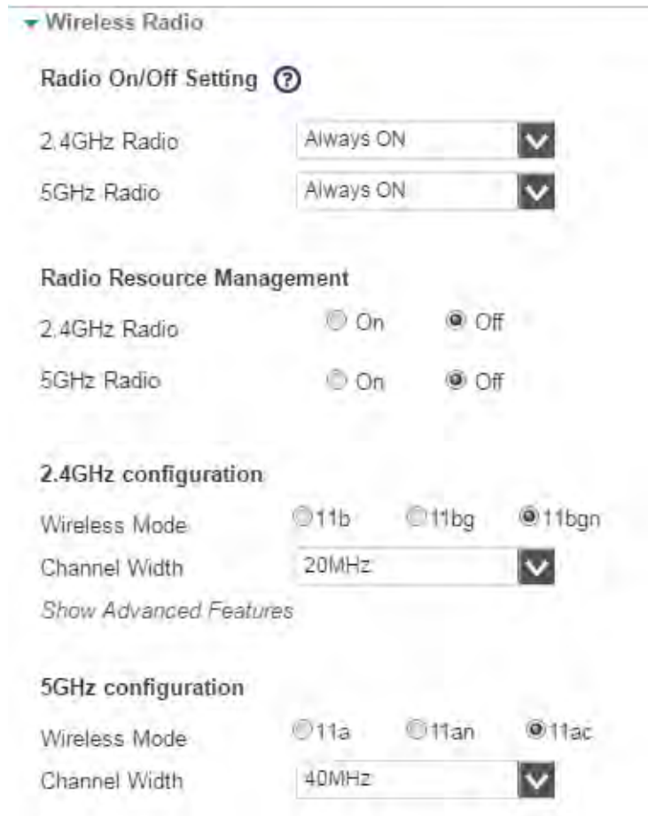
Figure 49. Expanding Wireless Radio Area
