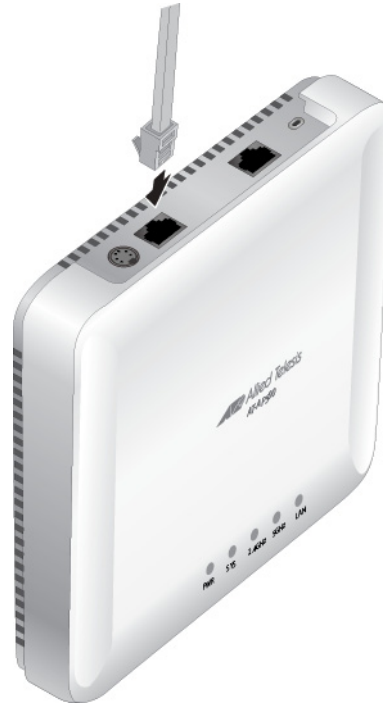
Figure 10. Connecting the Network Cable
