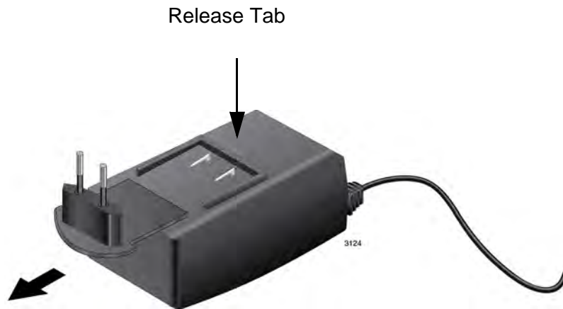
Figure 12. Removing an AC Plug from the AT-TQ0091 AC/DC Power Adapter
