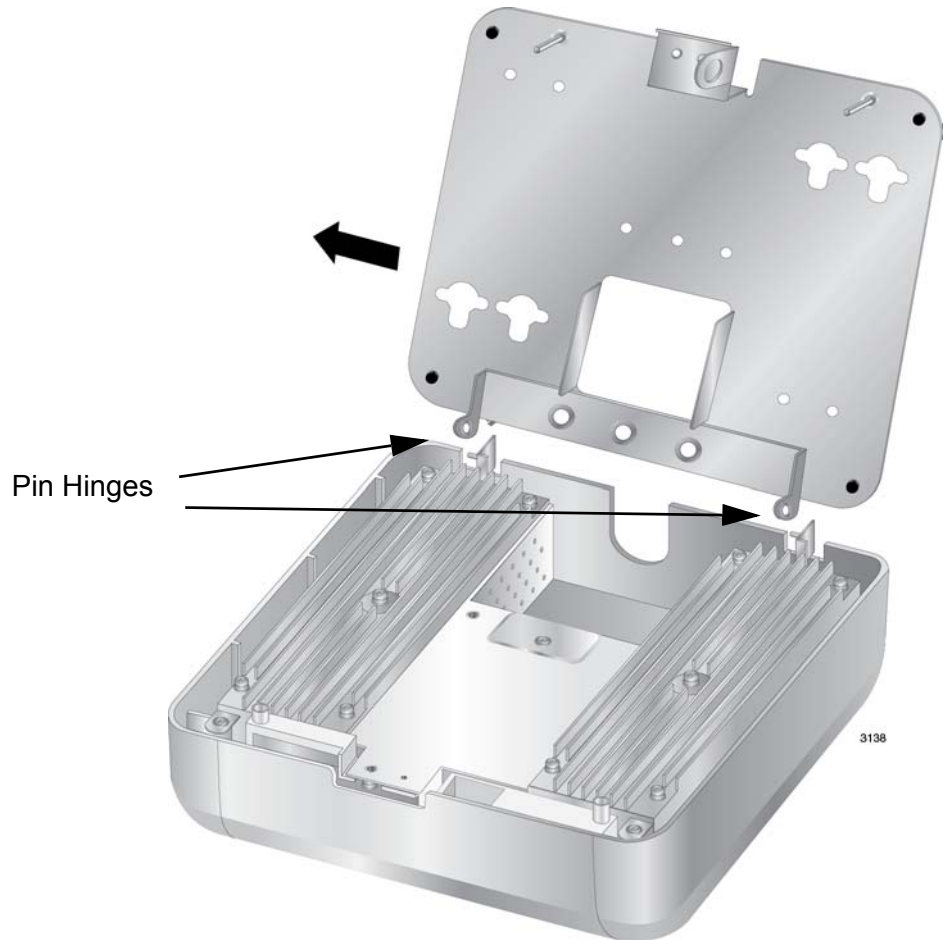
Figure 16. Removing the Bottom Panel from the Wireless Access Point
