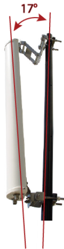
Figure 6. AT-AN5158-16DP Sector Antenna Adjustment
