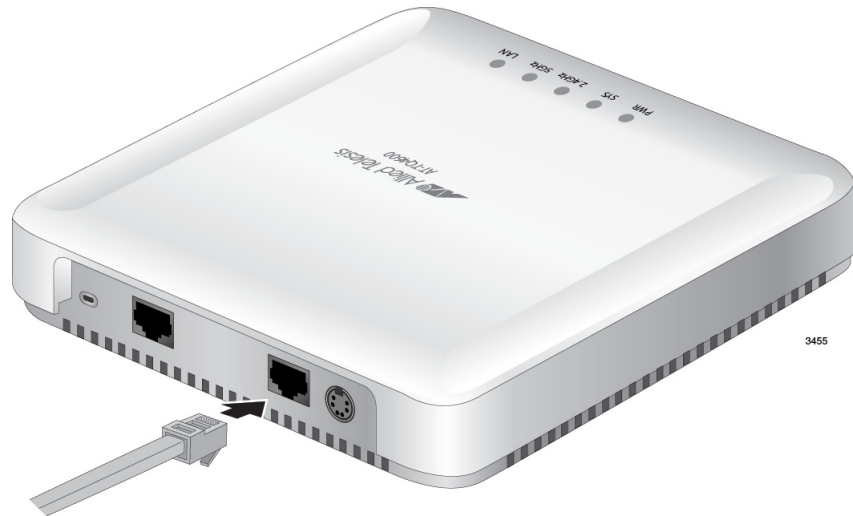
Figure 4. Connecting the Network Cable for Table or Desktop Installation
