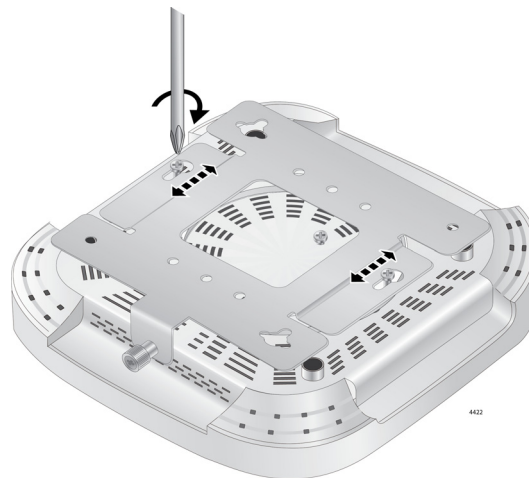
Figure 6. Adjusting the Screws on the Access Point
