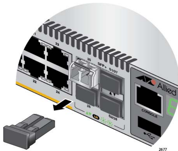
Figure 26. Removing the Dust Cover from an SFP or SFP+ Transceiver
