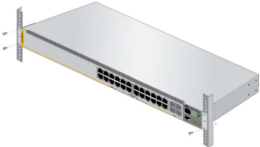
Figure 18. Mounting the Switch in an Equipment Rack
