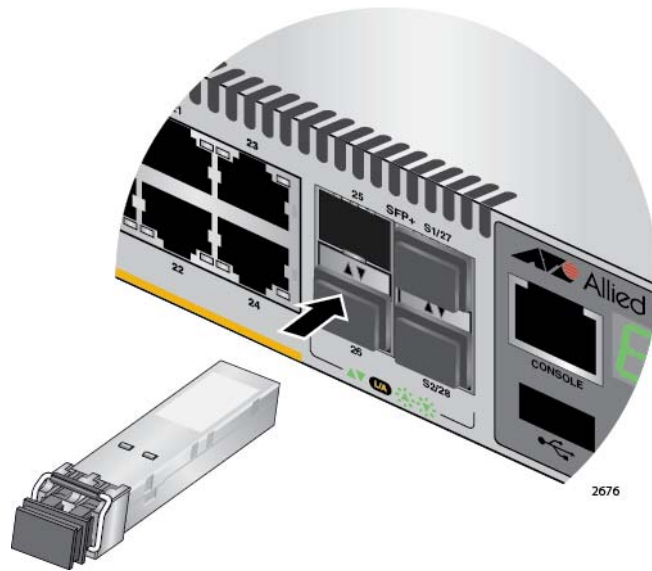
Figure 25. Installing an SFP or SFP+ Transceiver
