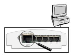
Push in the plug of the UTP cable into the LAN port until you hear a "click" and make sure it is correctly fixed by pulling the UTP cable lightly. In the same way connect the plug on the other end of the UTP cable to the network inteRFace card of the computer, or other LAN device.
