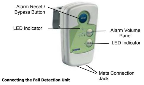
Plug the chair / bed /Incontinence mat into the mat connection jack, ensuring that the cable between the mat and the Fall Detection Unit can move freely and is clear of any moving parts.
