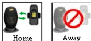
When the 1 Piece (Gen 4) is in range of the Beacon, it will start receiving signals from the Beacon and will record a “Home” status. The 1 Piece (Gen 4) will remain in the “Home” status until it is taken out of range of the Beacon.
