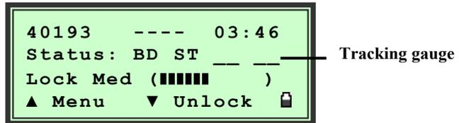
You can use the displayed visual tracking gauge to estimate the approximate distance between the Mobile Unit and the selected Offender’s Transmitter.
