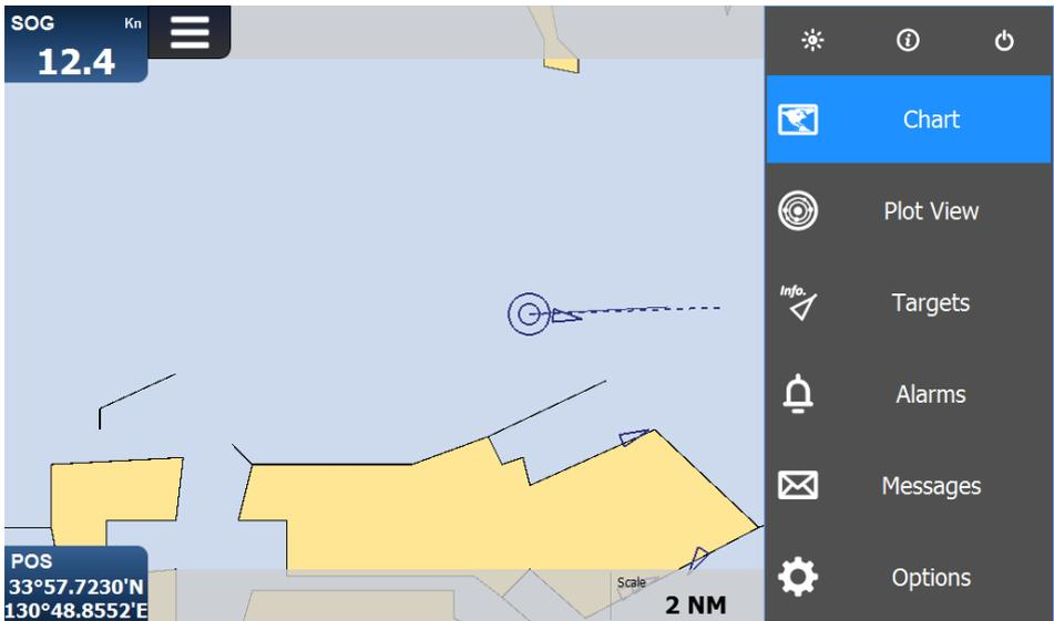
The P200 contains an application which will display AIS targets received, along with its own vessel position on a basic world chart by default. It supports the C-MAP 4D to provide more detailed and high-resolution charts which can be purchased separately by C-MAP dealers. The basic chart operations:
