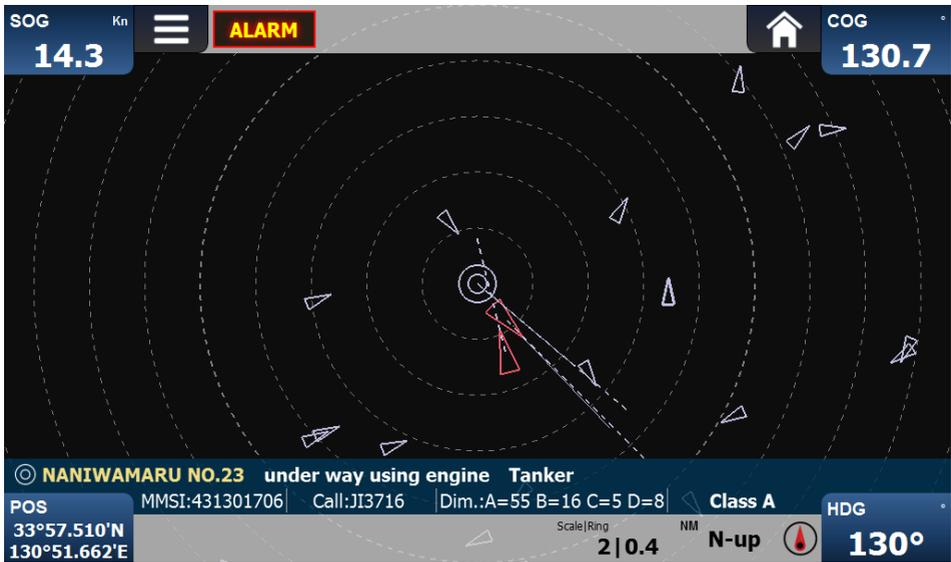
Plot view is the screen to show the location of other AIS targets relative to your own vessel. The own vessel's static data is displayed on the blue bar. The plot range from 0.1NM up to 1000NM can be adjusted by pinching the touch screen or pressing the zoom-in or zoom-out buttons. In Plot view's menu, the 3 different orientation modes can be selected.
