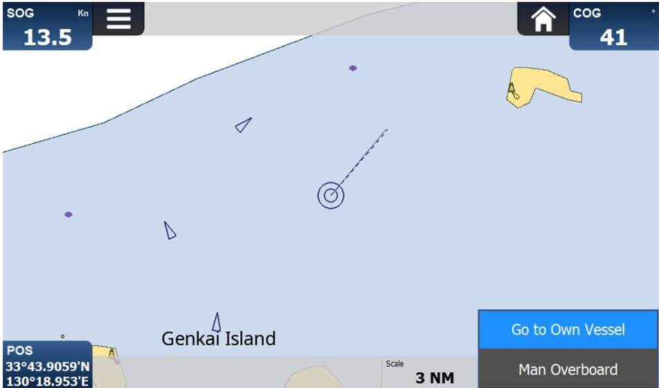
When pressing the Fn Key and select “Man overboard”, you can create a Man Overboard (MOB) for an emergency. This means:
