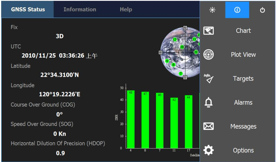
The Device Information can be accessed by pressing on the
