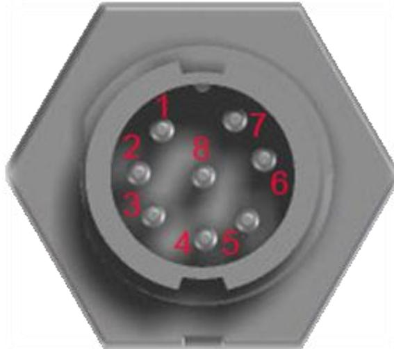
**Figure 3-2 Pin Assignments Front View**
