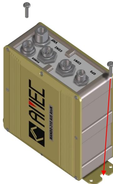
Figure2-2-4 Installation: Vertical Type
