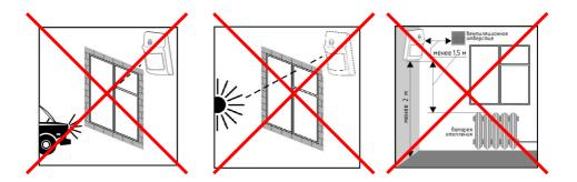
The wall with motion detector shouldn't receive heavy vibration.
