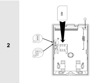
Insert the SIM card into its holder. Set the jumper in position 1 or 2.
