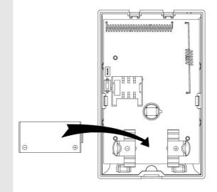
Insert the battery into the motion detector slot observing polarity.
