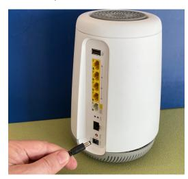
2. Plug the power adapter into a power outlet.
