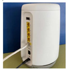
4. Plug other end of Ethernet cable into the CenturyLink support connections (ONT) or wall jack.
