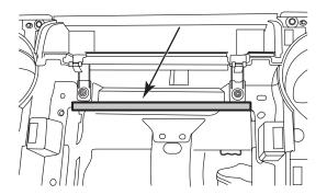
3 Connect the factory harness to the main harness and secure it.
