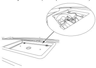
5 Access the ODBII connector located under the driver side dashboard. Connect the YELLOW/BROWN wire from the Alpine harness to the WHITE wire located at pin 14 of the OBDII connector. Connect the RED/ BROWN wire from the Alpine harness to the WHITE/ BLUE wire located at pin 6 of the OBDII connector.
