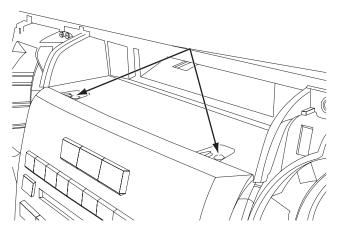
7 Extract 4 x 7 mm screws from the factory radio and remove it.
