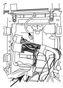
Only use if vehicle is equipped with a factory subwoofer and harness was plugged into the OEM headunit.
