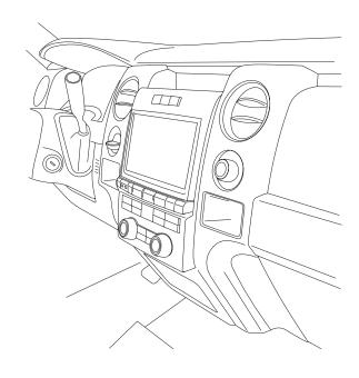
2 Install the HVAC control and Hazard light switch on to the G-KTX-009-F150 panel.
