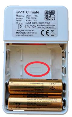
Note polarity symbols in the battery compartment
