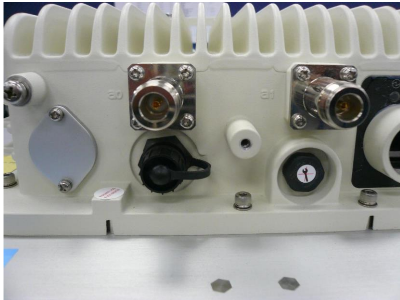
Figure 22. 5GHz "a0 & a1" antenna RF ports
