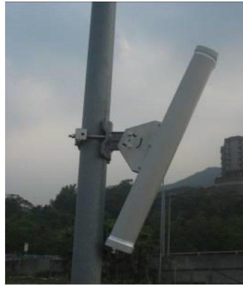
Figure 18. Adjust A8n (ac) 2.4GHz Antenna tilting
