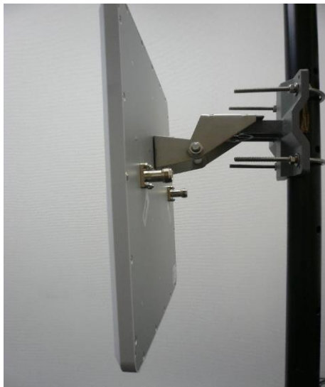
Figure 23. 20dBi 5GHz Antenna mounting
