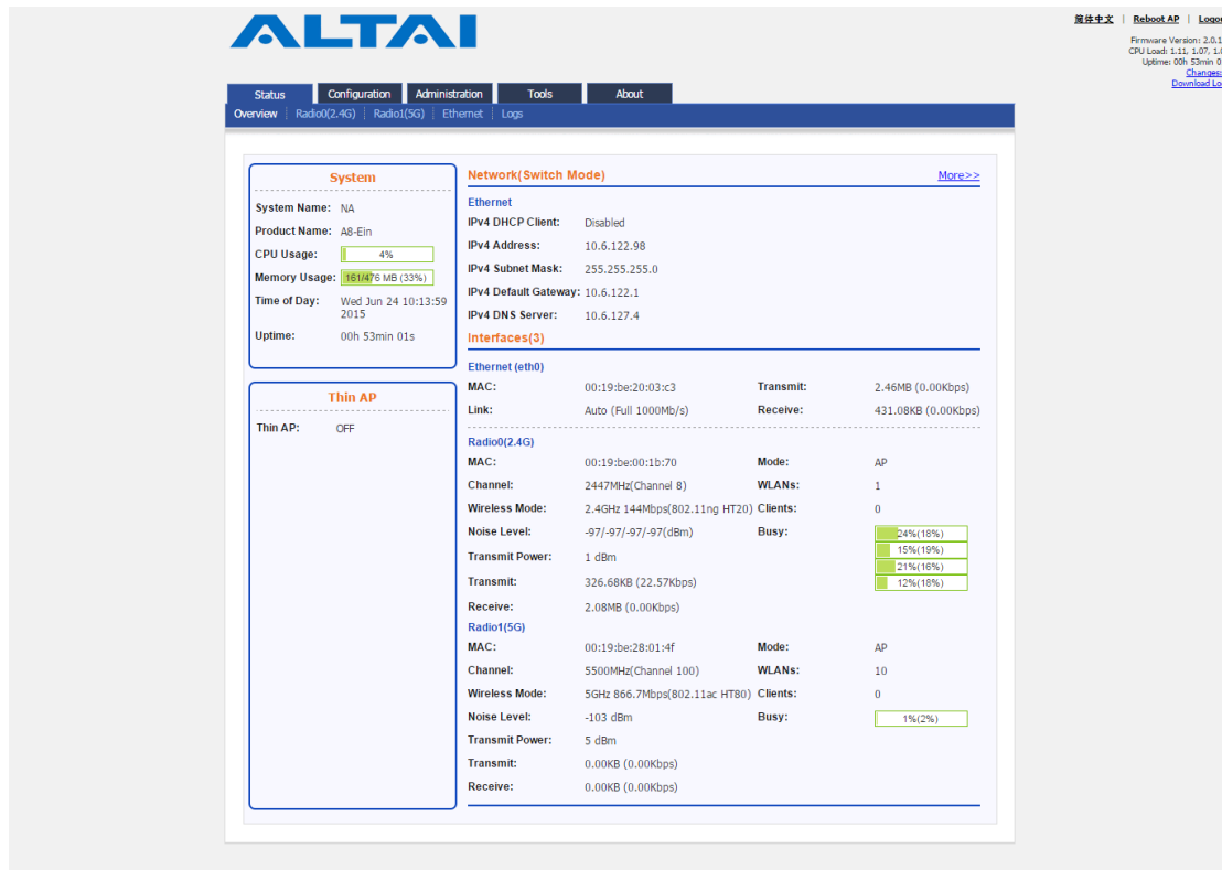
Figure 4 – AP Status Overview
