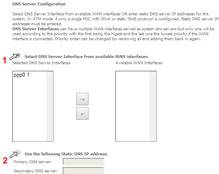
Figure 53: WAN Service setup – DNS Server configuration window
