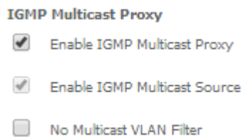
Figure 51: WAN Service Setup – Connection establishment configuration window- IGMP Multicast Proxy configuration
