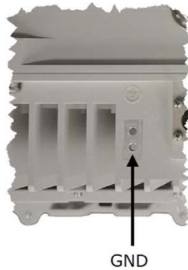
Figure 3-5 iRM2249 iRRH ground connector location
