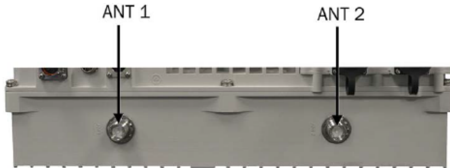
Figure 3-2 iRM2249 iRRH RF connectors location
