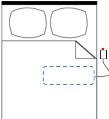
4. Release the mattress, allowing the weight of the mattress to be applied to the pad.
