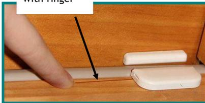
Run a light coat of permanent paste glue on the underside of the antenna
