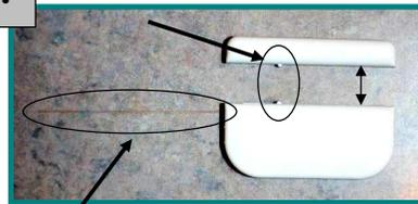
Position Antenna free and clear of sensor; not inside cover or under sensor.
