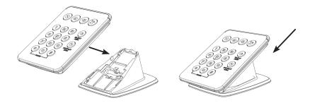
4. Coil up the excess power wire into the stand. Insert wire into wire holder and close stand cover to contain excess wires.
