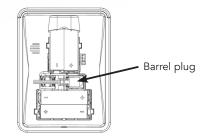
4. Insert the Keypad into the mounting plate. Push any extra wire behind wall plate before inserting into mounting plate. Slide the Keypad on plate until it "clicks" into place.
