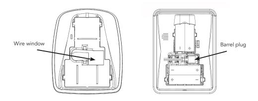
3. Insert the Keypad into the table stand. Push any extra wire into stand before inserting into stand. Slide the Keypad on stand until it "clicks" into place.
