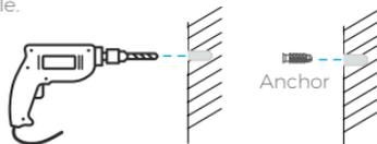
5 Fix the mounting plate to the wall.
