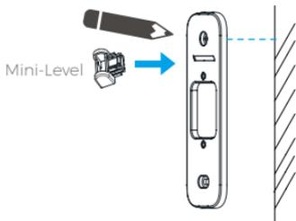
**i** Remove the mini-level when drill points are marked.
