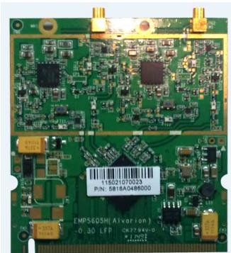
Alvarion miniPCI series radio modules perform extreme high power and economize the power consumption on the system platform. **EMP5605H (ALVARION)** is an 802.11a/n WiFi 2x2 mini-PCI module designed specifically for integration to maximum performance ratio. EMP5605H (ALVARION) delivers the ultimate wireless triple play experience for video, voice, and data transmission in the home, for the business, and on the road.
