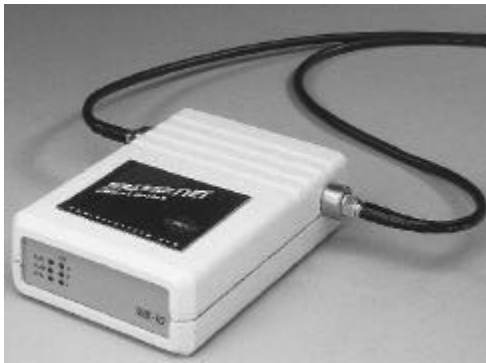
Figure 1.1: WB-10D PRO.11 with Two External Antenna Connector Ports
