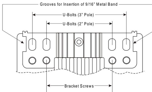
**Figure 2-1. Holes/Grooves/Screw Holes**
