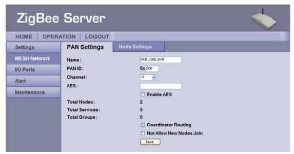
PAN Setting: input or modify ZigBee network setting.
