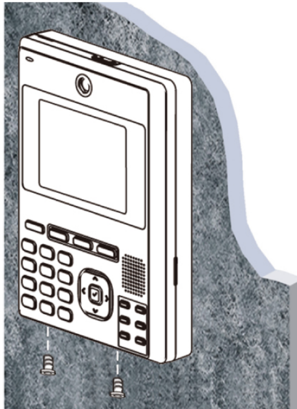
Screw the Video Indoor Station with Back Plate wall
