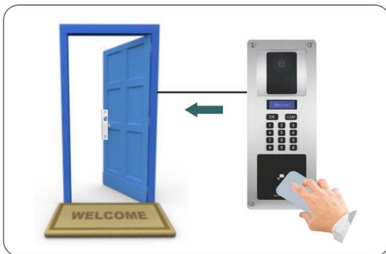
Figure 33: Scan RFID card to open door
