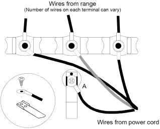
A—Ground screw (Connect green insulated wire and secure with screw.)
