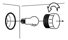
Replacing Oven Light Bulb
