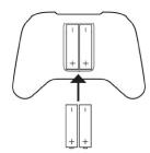
Remove the battery compartment cover and insert the batteries\*. Be sure to orient the positive (+) and negative (–) ends as shown on the compartment labels.
