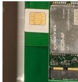
3. Push the SIM card into the connector using a suitable plastic tool.
