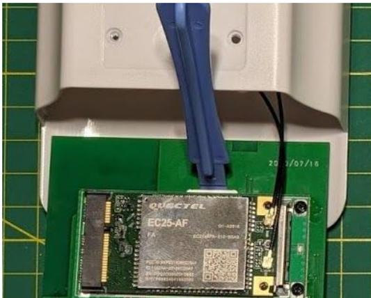
4. Slide the electronics assembly back into the case being careful to prevent damage to internal components or antenna cables.
