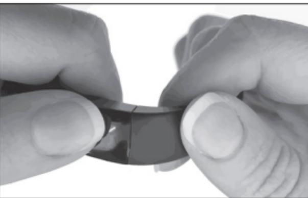
2. While firmly holding, gently pull the wrist strap away from the tracker module to remove.
