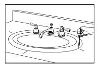
Connect supply line to faucet (finger tight) and carefully bend tubes to engage with the supply shut-off valves. Tighten connections at faucet and shut-off valves for secure seal.
