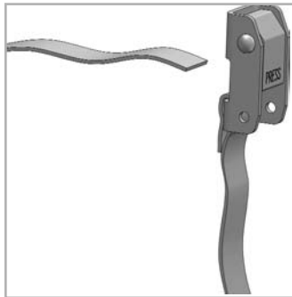
1. Thread tag end of STRAP up through hole in underside of BUCKLE.
